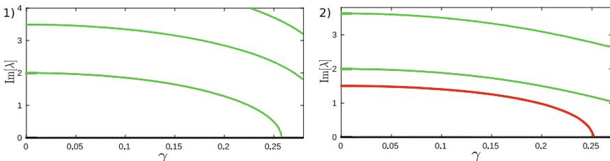
**Fig. 3** Purely imaginary eigenvalues  $\lambda$  of the  $\mathcal{PT}$ -symmetric problem (30) for the first two stationary states with  $\mu = 12$ . Eigenvalues of negative (positive) Krein signature are shown in red (green), complex eigenvalues are shown in black
