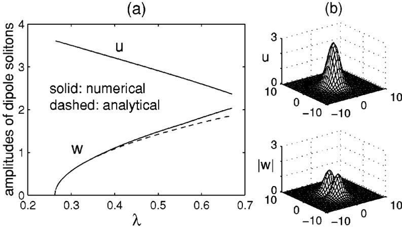
FIG. 3. (a) Amplitudes of the dipole vector solitons obtained analytically (dashed line) and numerically (solid line) for  $s=0.5$  and various frequencies  $\lambda$ . (b) A numerical dipole-soliton solution with  $s=0.5$  and  $\lambda=0.5$ .
